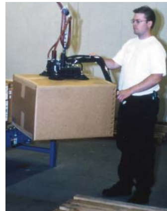
Vacuum lifters make the handling of large or heavy containers easier.
